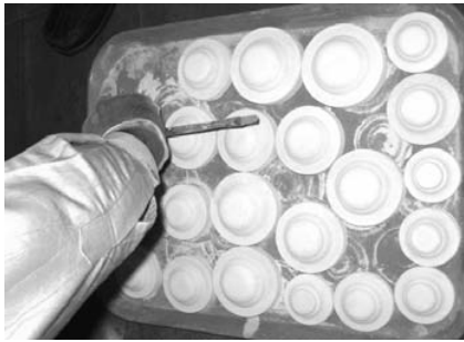
Fig. 5. Printed and cleaned shells.
