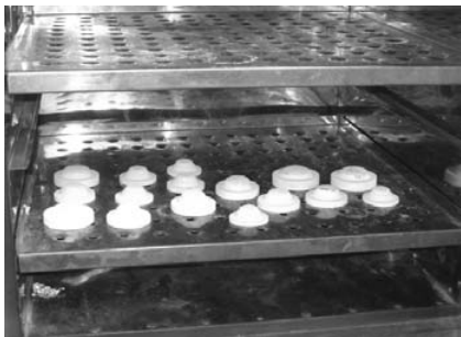
Fig. 6. Post curing of shells by heating at 110°C for 1 hour.
